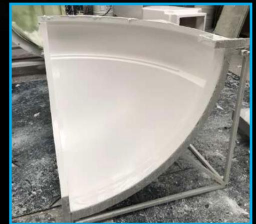
■ The moulds Pulsar use to fabricate the domes.
